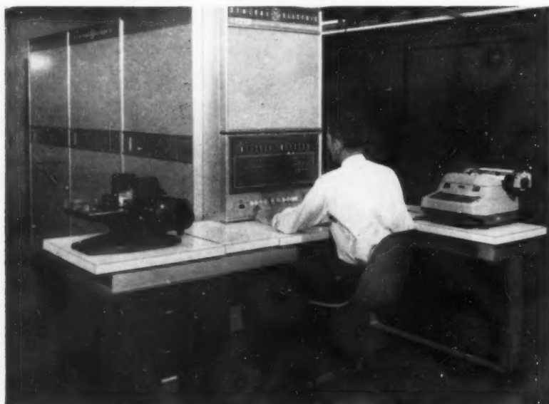
GE-225 is a medium-priced, general purpose computer made by the General Electric Company that can be used for scientific applications as well as complex business data processing. This all-transistorized system automatically translates English words and symbols into machine language thus expediting programming techniques.
